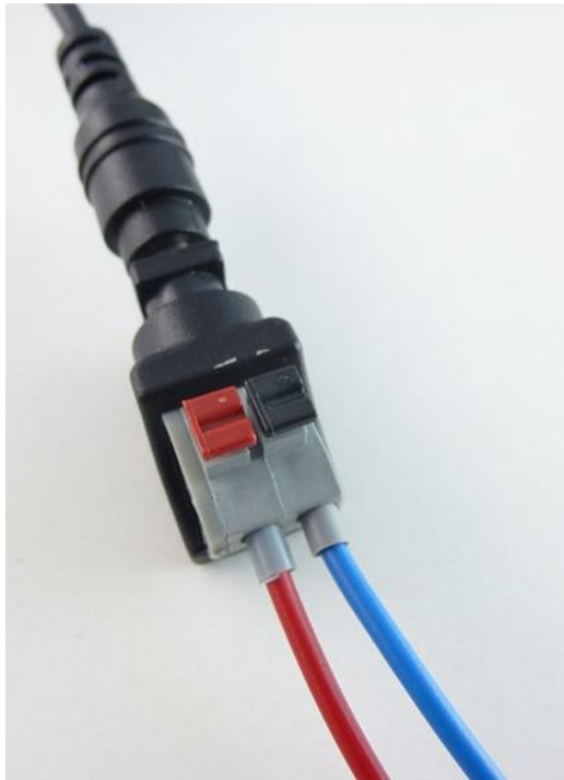
Figure 34: Wire connection to the adapter
