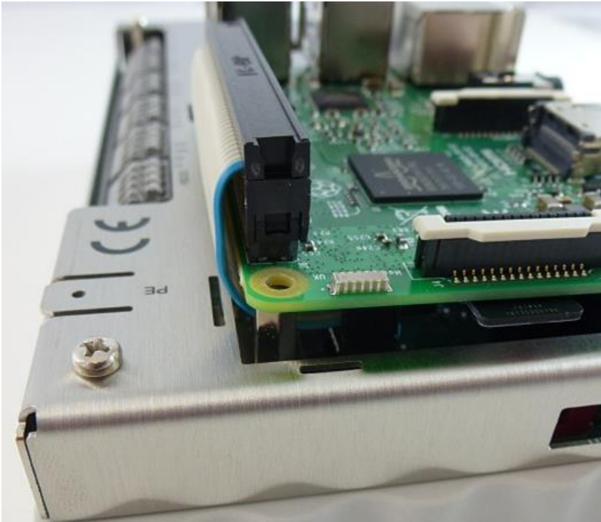
Figure 23: Optimal routing of the ribbon cable
