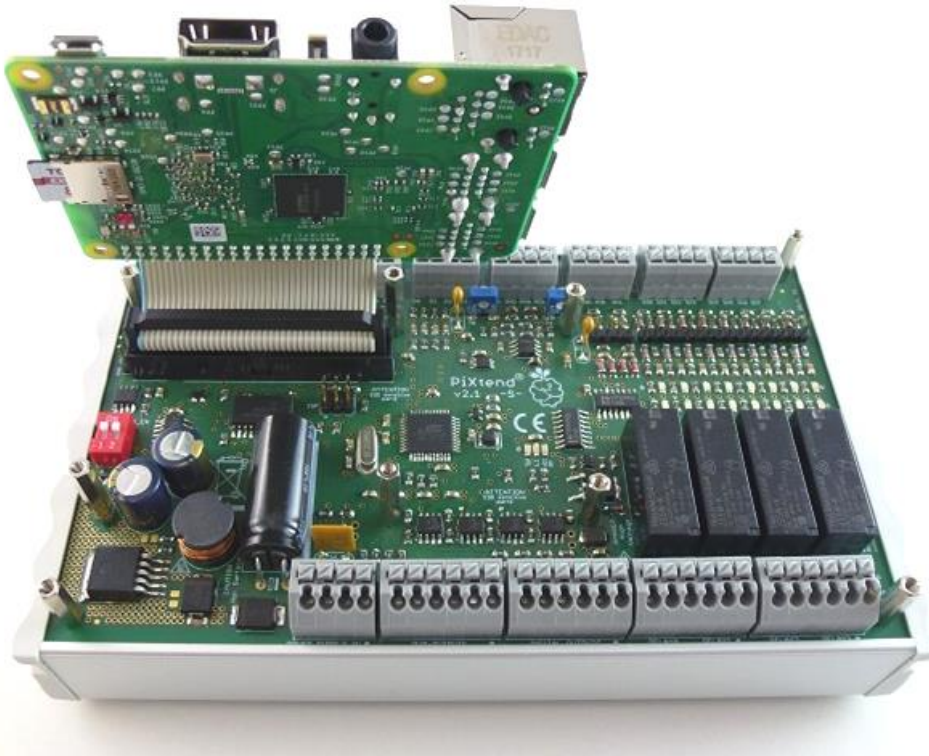
Figure 19: Raspberry Pi unscrewed from the PiXtend (ribbon cable remains connected)
