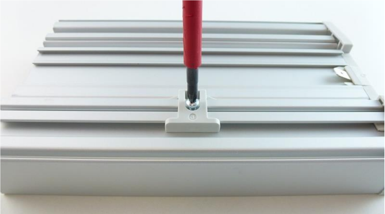
Figure 12: Screwing the locking bracket into place
