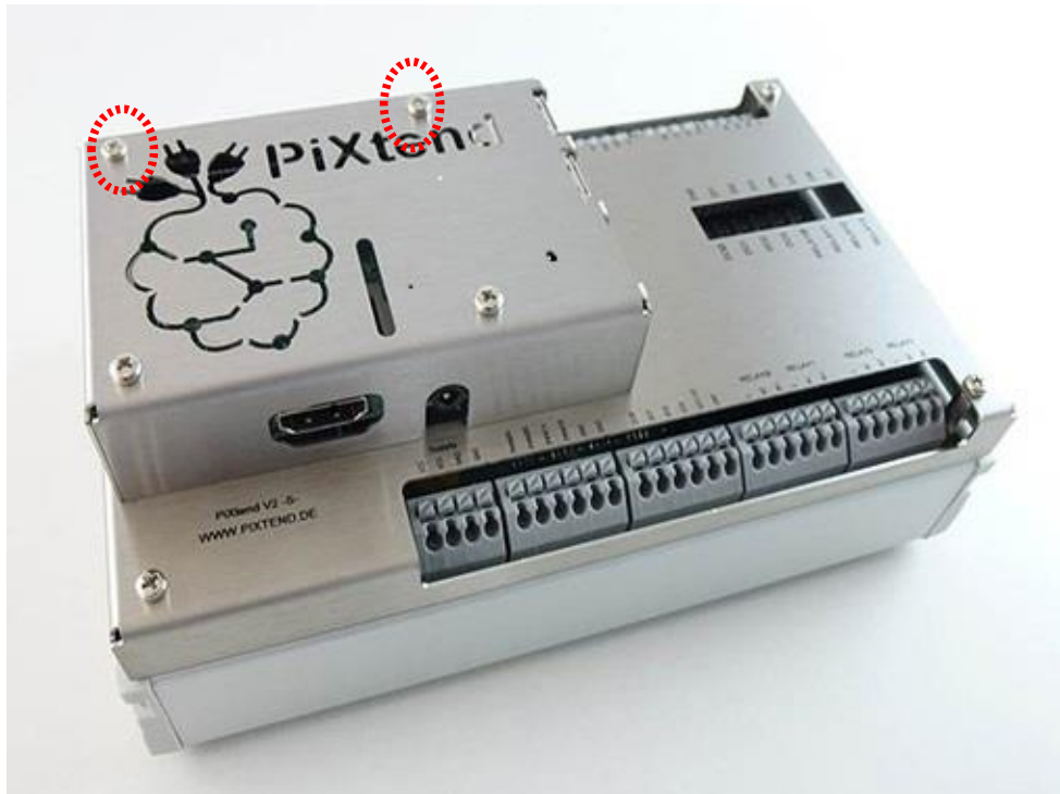
Figure 26: Completely assembled stainless-steel cover
