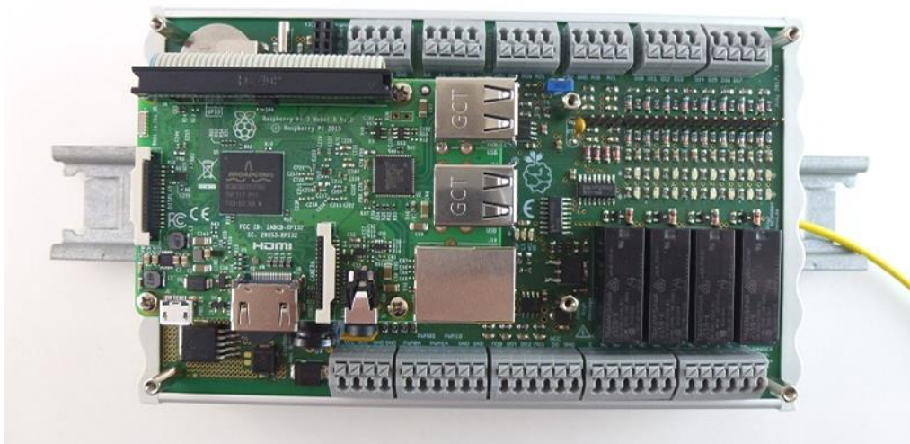
Figure 18: Completed DIN rail mounting
