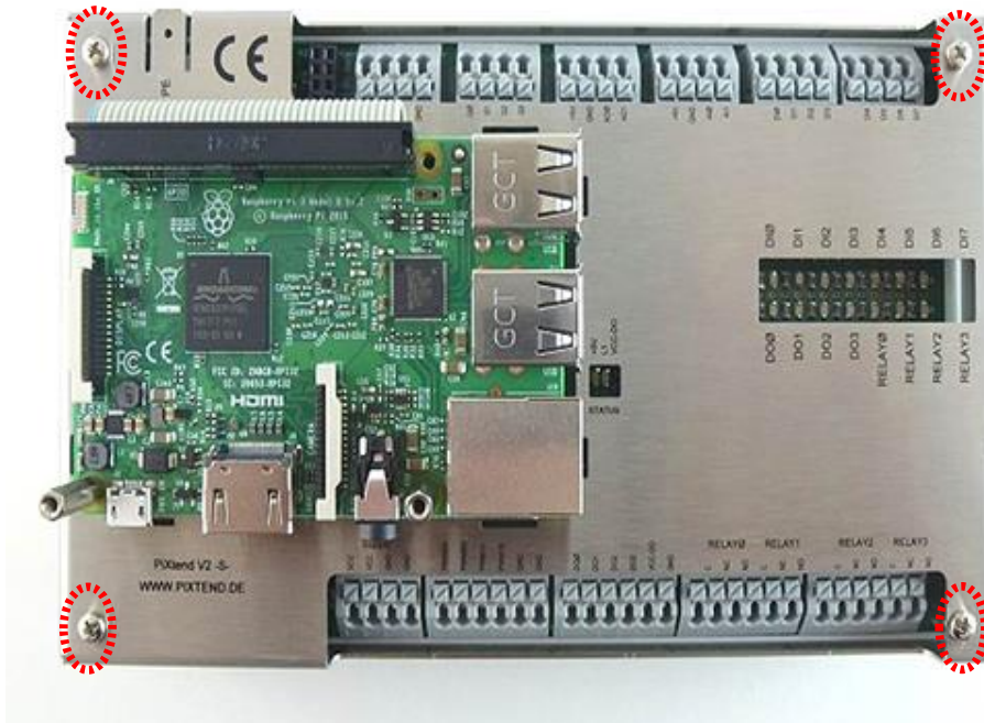
Figure 22: Screw points for the lower part of the cover
