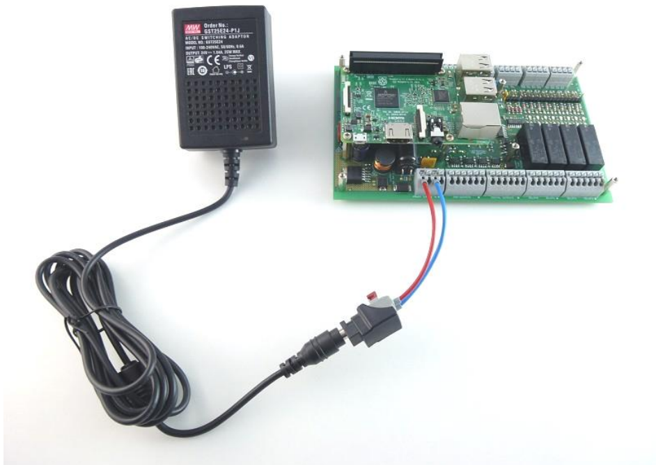
Figure 36: Power supply connected to the PiXtend V2 -S-
