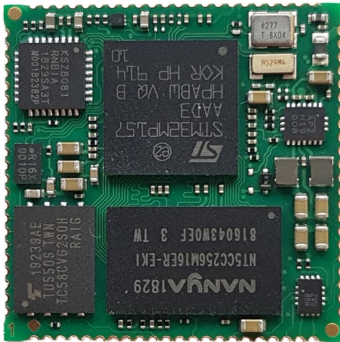
Figure 1: 25,5x25,5mm SoM with castellation and LGA Pads
