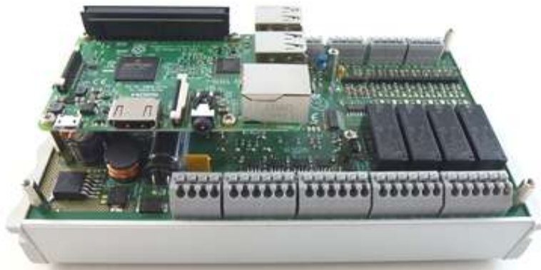
Figure 14: Assembled DIN rail housing
