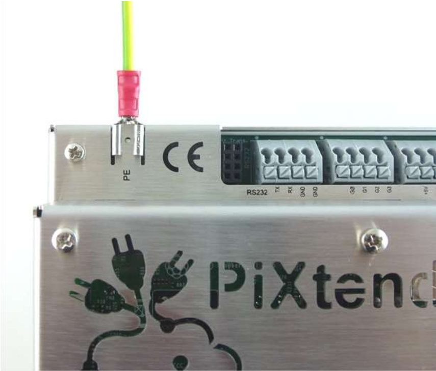
Figure 27: Grounding connection (PE) on the PiXtend V2 -S- cover
