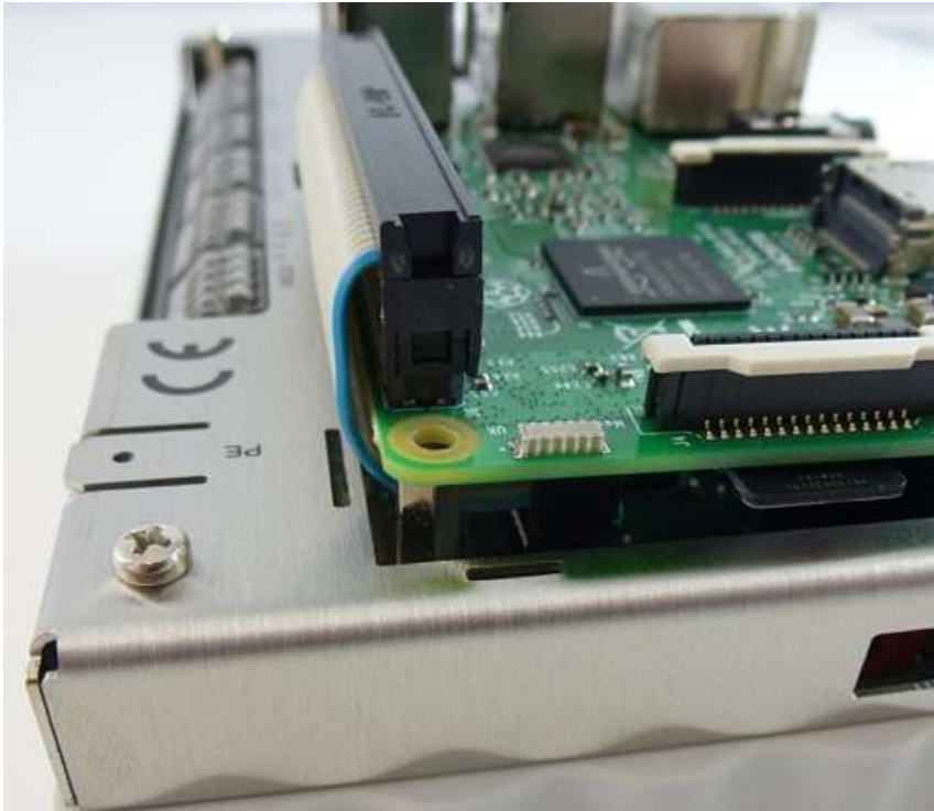
Figure 23: Optimal routing of the ribbon cable
