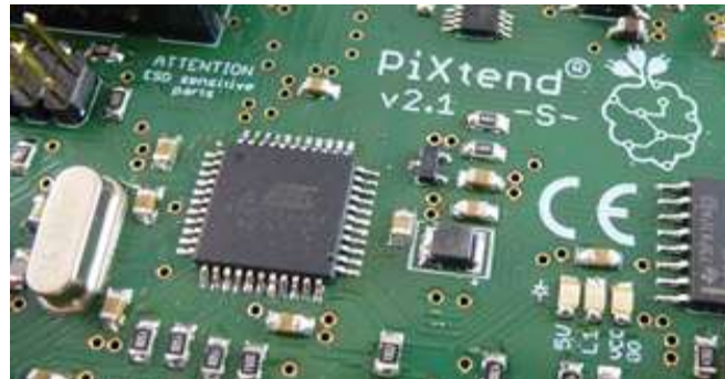
Figure 46: PiXtend V2 -S- micro-controller
