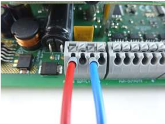
Figure 35: Power connection to the PiXtend V2 -S-
