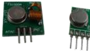
Figure 74: Typical inexpensive 433 MHz transmitter
