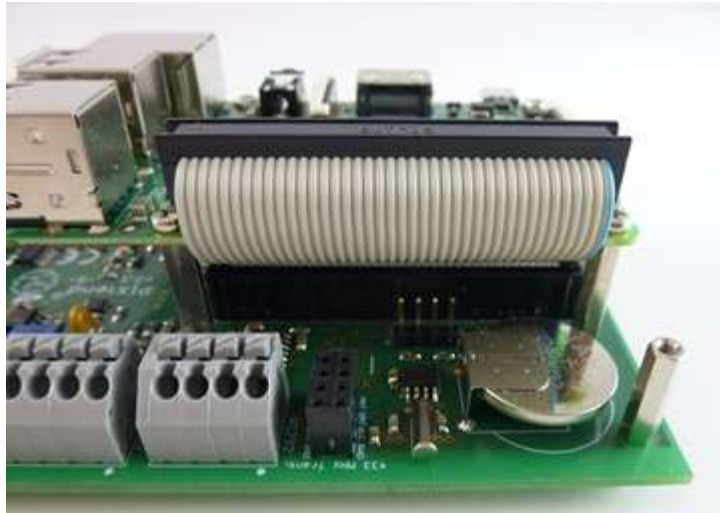
Figure 41: Connection between the PiXtend V2 -S- and Raspberry Pi
