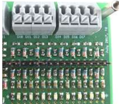
Figure 52: Terminal block - digital inputs
