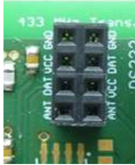
Figure 73: Two-row socket connector for 433 MHz transmitters
