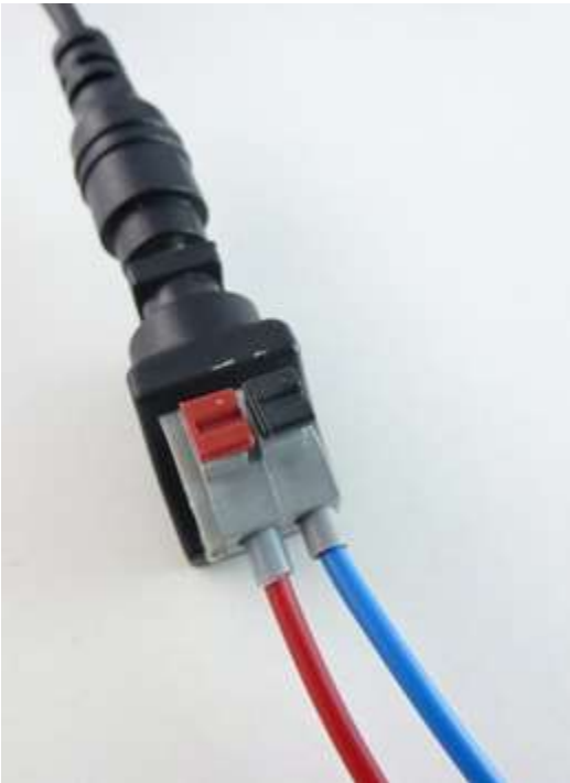
Figure 34: Wire connection to the adapter
