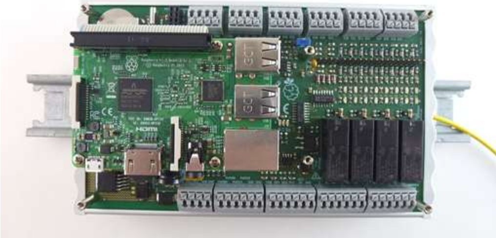
Figure 18: Completed DIN rail mounting
