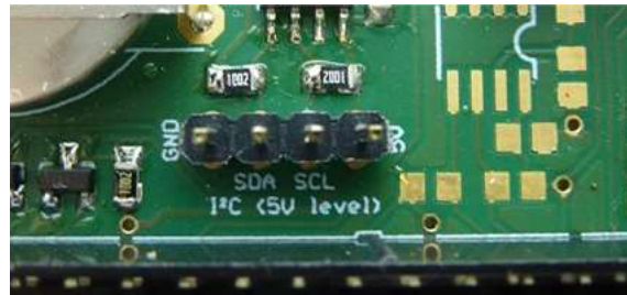
Figure 43: Pin header - I 2 C on 5V level
