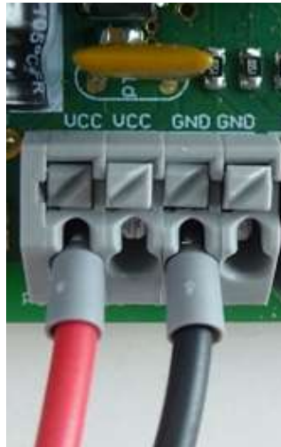
Figure 39: Terminal block for the power supply
