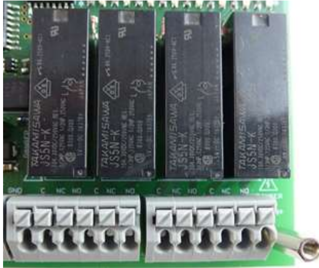
Figure 57: Terminal connection block – relay
