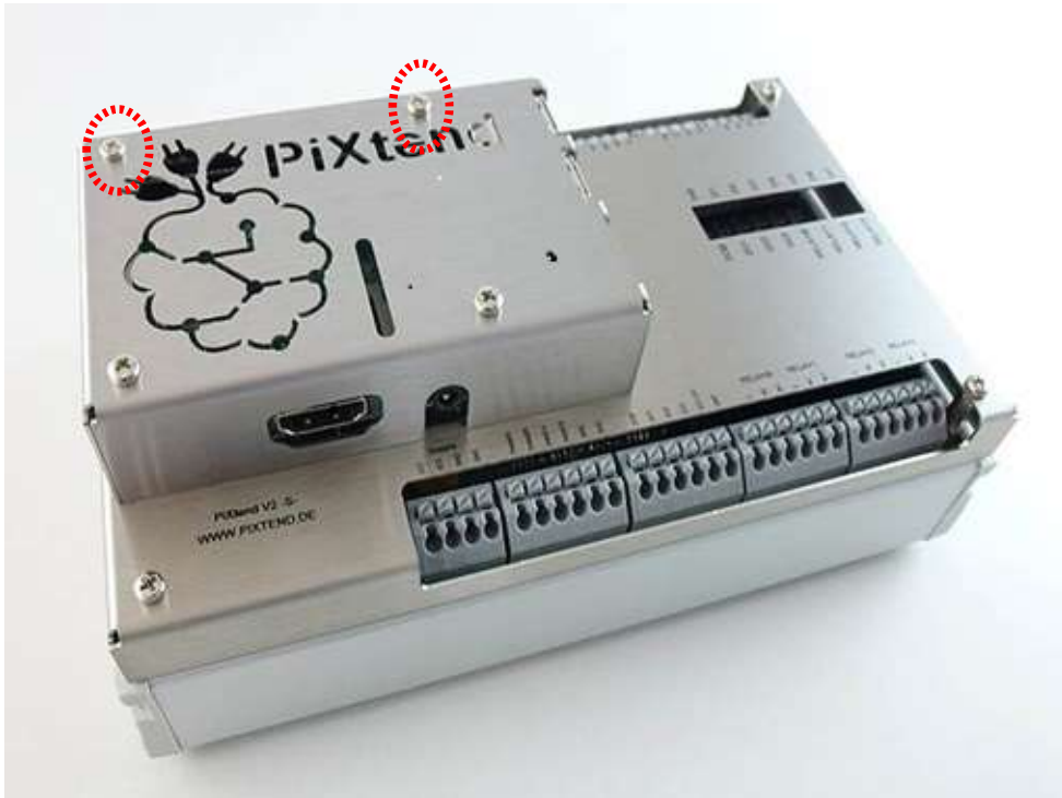
Figure 26: Completely assembled stainless-steel cover
