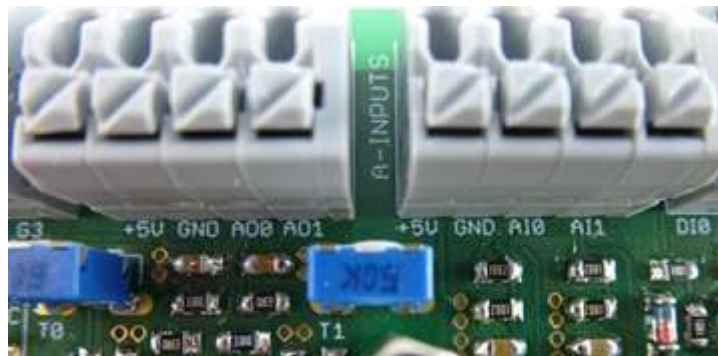
Figure 63: Terminal blocks - analog inputs and outputs
