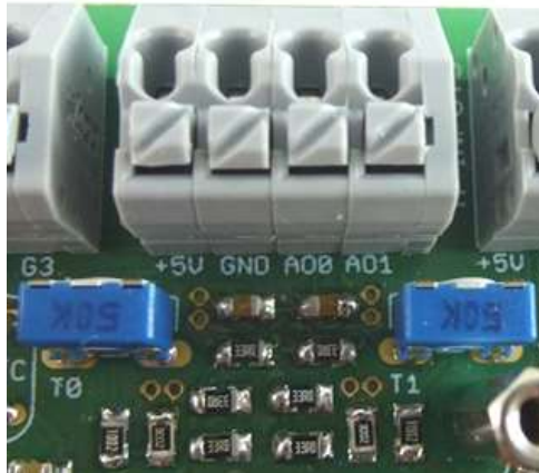
Figure 68: Terminal block - analog outputs
