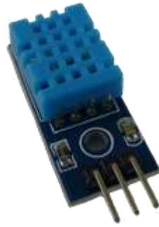
Figure 72: Temperature and humidity sensor DHT11
