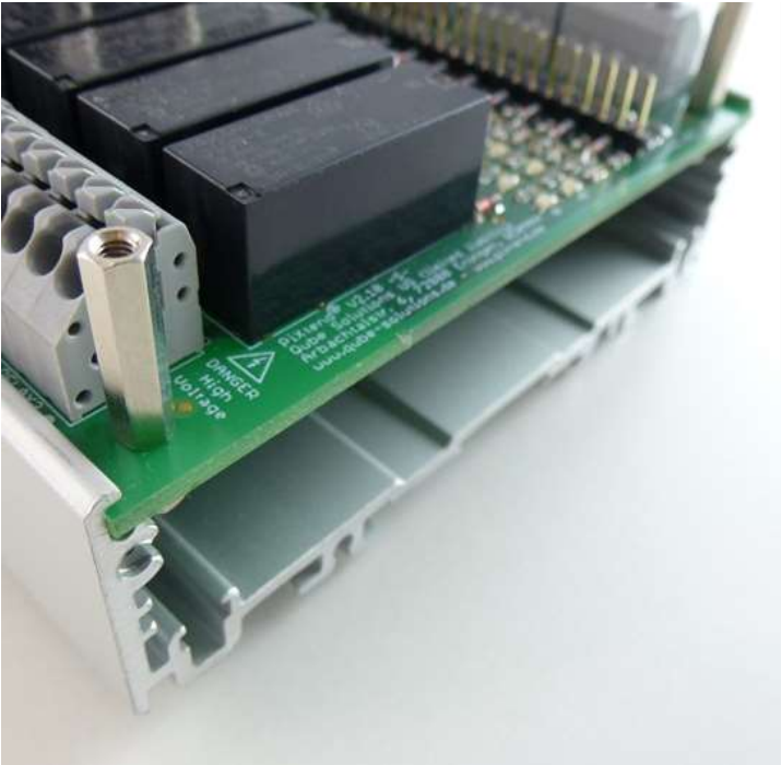
Figure 13: Connecting the PiXtend and housing profile together
