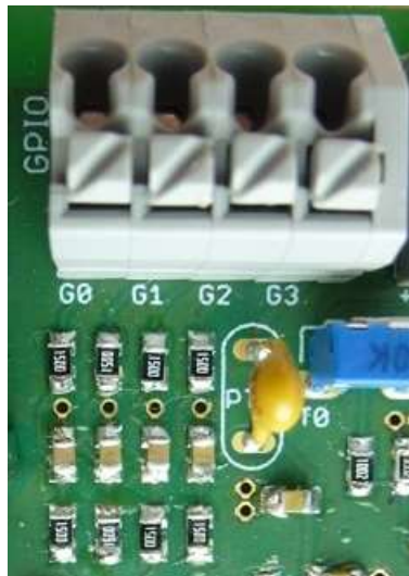
Figure 60: Terminal block connection - GPIOs
