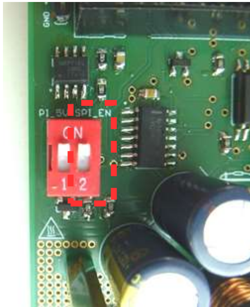
Figure 47: DIP switch: SPI_EN
