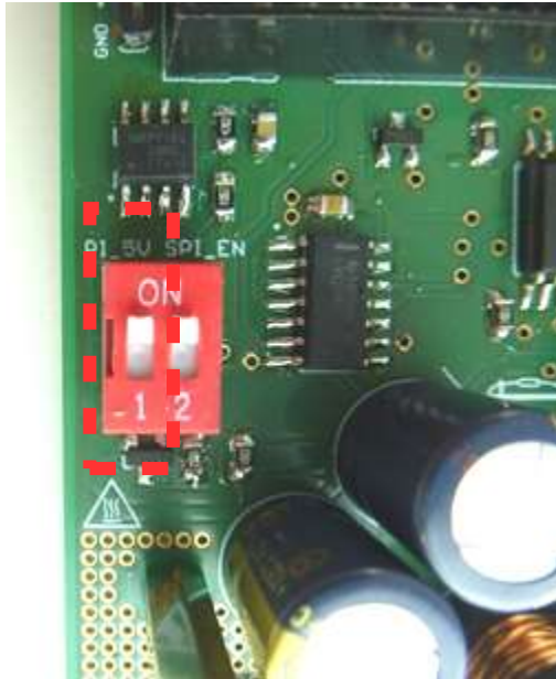
Figure 29: “PI_5V” in the “ON” position
