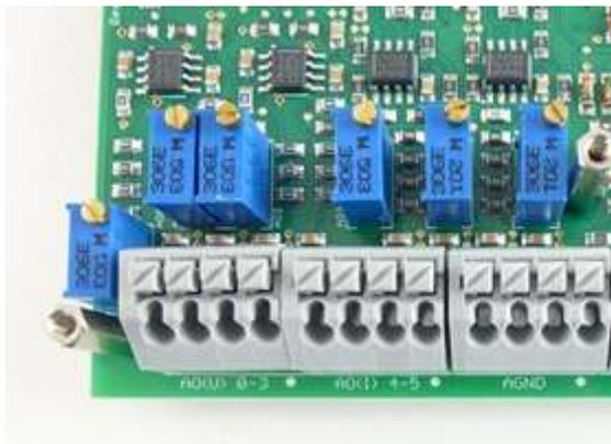
Figure 45: Terminal block – analog outputs
