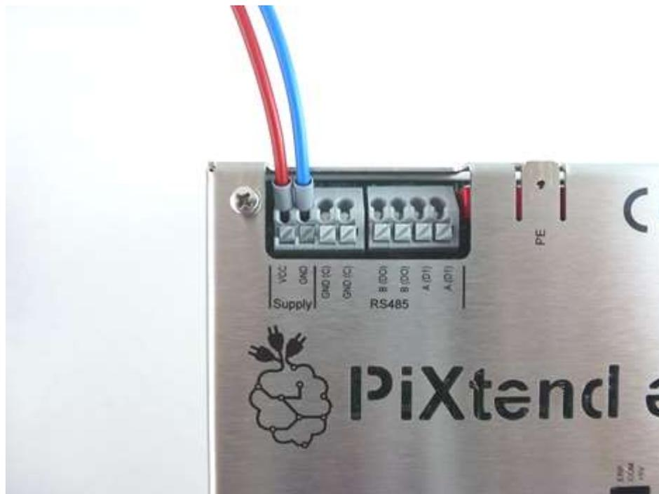
Figure 25: Power connection to the PiXtend eIO
