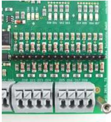
Figure 35: Terminal block - digital inputs
