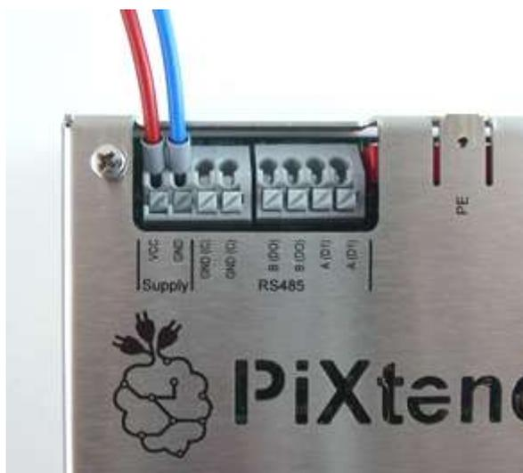
Figure 30: Terminal block for the power supply
