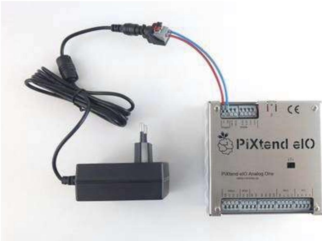
Figure 26: Power supply connected to the PiXtend eIO
